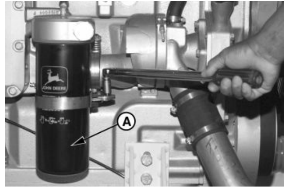
Replace Engine Oil Filter
