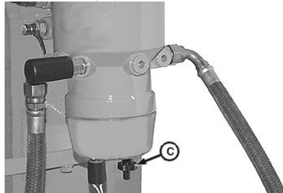
Draining Fuel Sediment Bowl (Earlier Engines shown)
